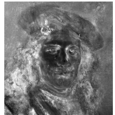
Fig 2. XRF scan of iron (FeK), detail of face, Man with a Sword , Geert van der Snickt (University of Antwerp) and Joris Dik (Technical University of Delft)
